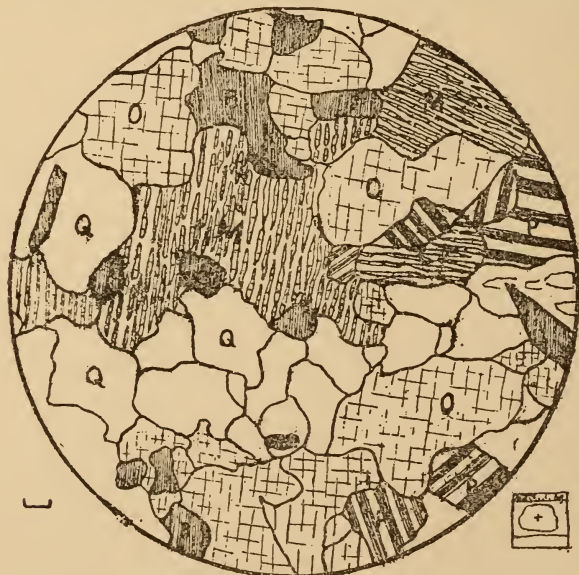
FIG. 1.—Common biotite-gneiss, Bulwagga Mountain, Moriah. O is orthoclase; M, microperthite; Q, quartz; B, biotite; P, plagioclase.
