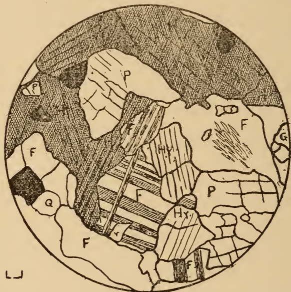
FIG. 2.—Gabbro without reaction rims—near Ensign Pond, Moriah. F is labradorite; P, augite; Hy, hypersthene; H, hornblende; Q, quartz; G, garnet; M, magnetite.
