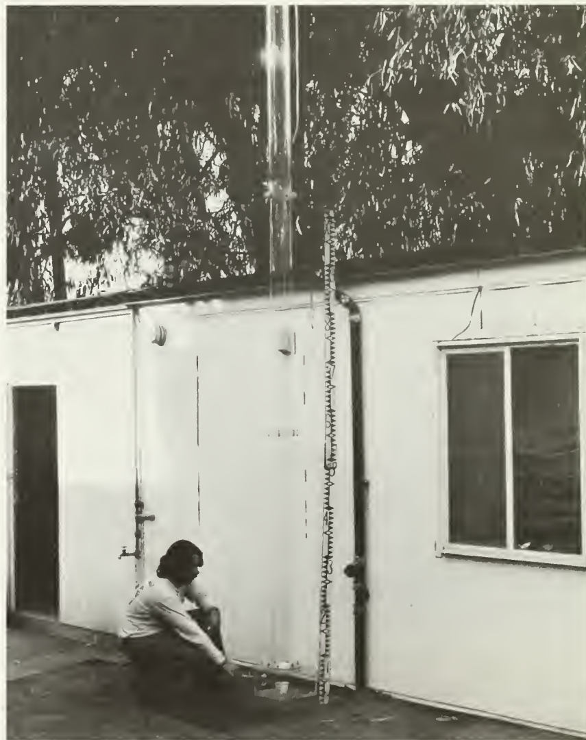
A 5-meter raindrop tower was used in trials to simulate rain impact.
