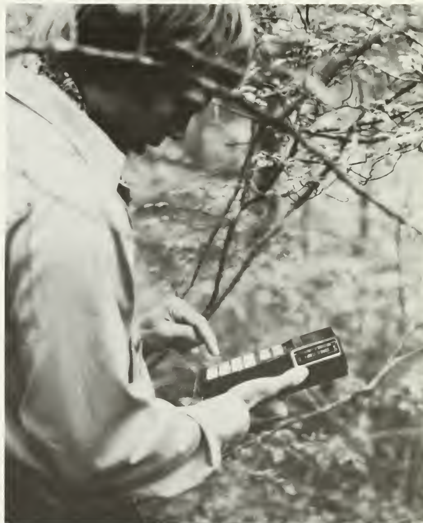
Electronic data recorders are used to collect timber stand data in Southern Forest Experiment Station surveys.
