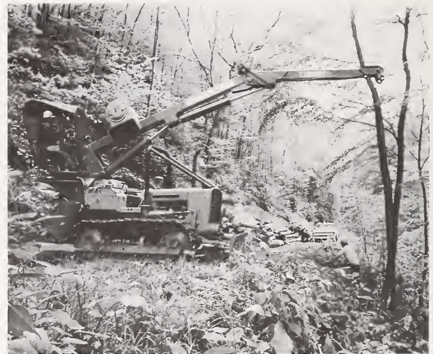
This new cable yarder can be used efficiently and economically on small woodland properties.
