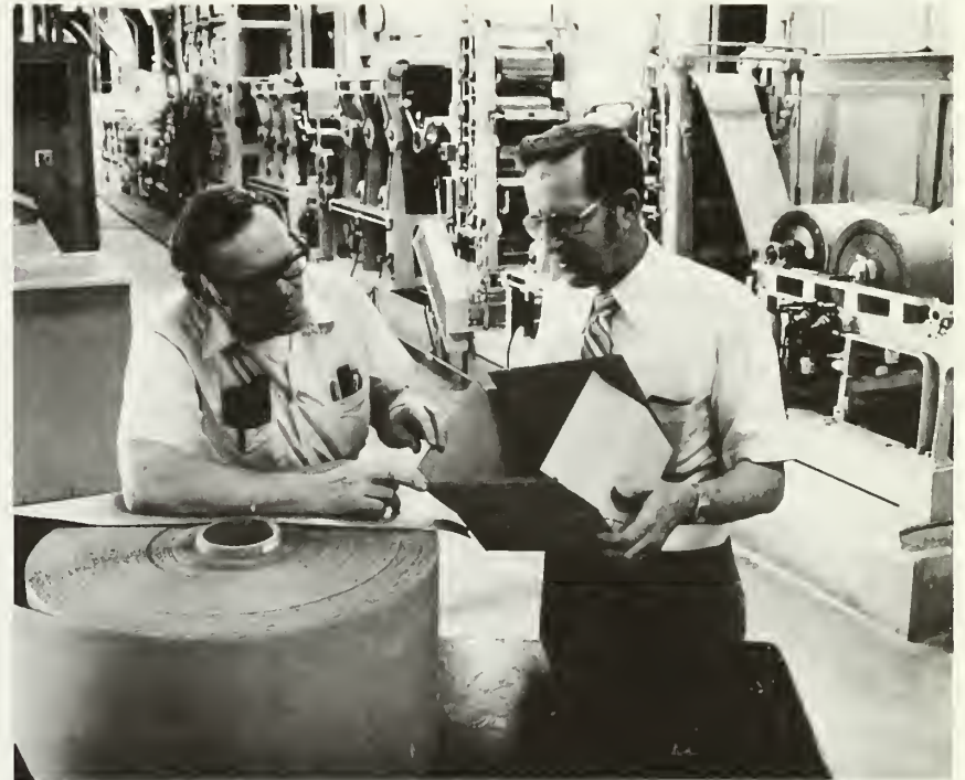
Researchers examine a sample corrugated fiberboard box made from 100-percent hardwood (red oak) pulp.
