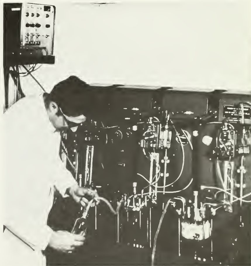
A fermentor is used in the production of improved Bt strains.
