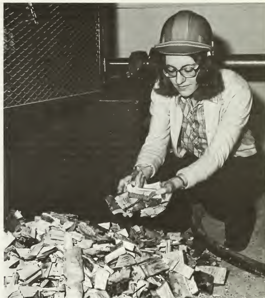
Spiral-headed chipper produces chunks instead of chips, which may be better for flakeboard and fuel.
