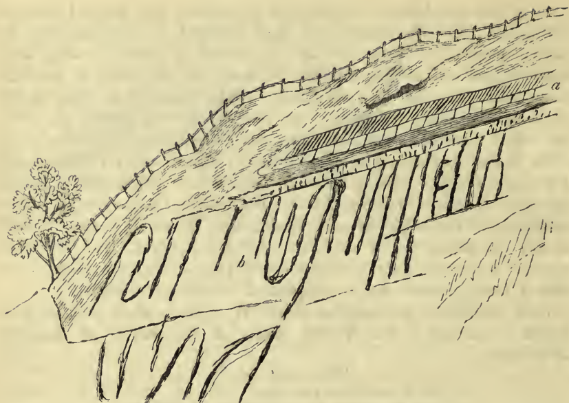
Section as seen from the opposite side of the ravine, about one hundred feet high. a , unconformable beds of Old Red Sandstone; b , vertical beds of Silurian strata. These beds of the Old Red are the finer quartzose Sandstone.
