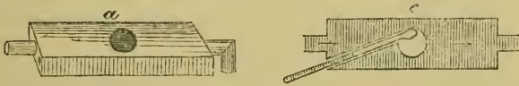
FIG. 1.— a . View of warm stage with inlet and outlet tubes, unconnected with heating apparatus. c . Horizontal section of stage, showing the manner in which the thermometer is passed into the central chamber, and the direction of the current of water in the stage.
