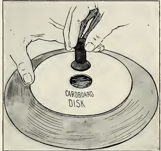
DISK SERVING AS GUIDE IN FASTENING SPOOLS.
