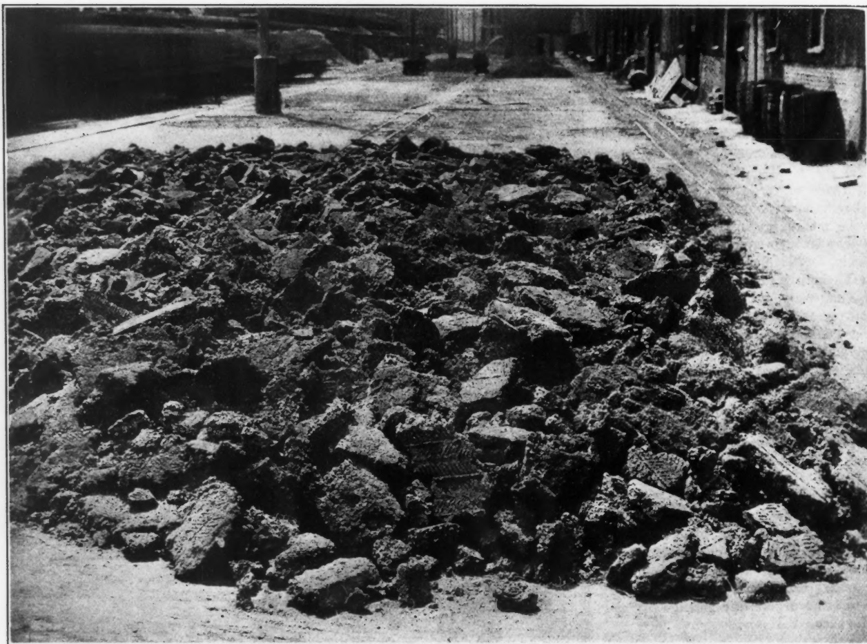
FIG. 2. SINTER CARRYING 50 PER CENT. LEAD MADE FROM GALENA CONCENTRATES, WITHOUT LIME
