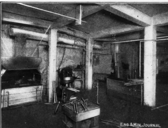
THE OTHER END OF THE SHOP. COKE FORGE ON LEFT, OIL FORGE AT RIGHT
