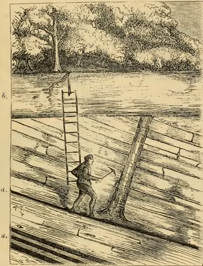
a, a. Coal-seams. b. Superficial Drift.
