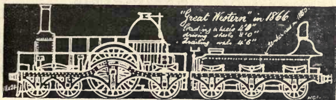
FIG. 35.—THE ORIGINAL "GREAT WESTERN" AS REBUILT WITH TWO PAIRS OF LEADING WHEELS
