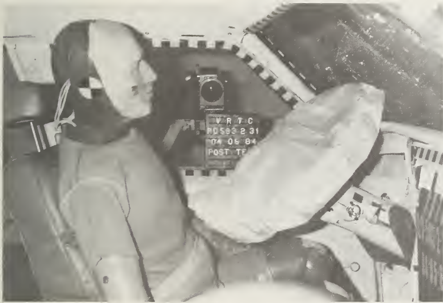
Test 31, Bag Position Post test
