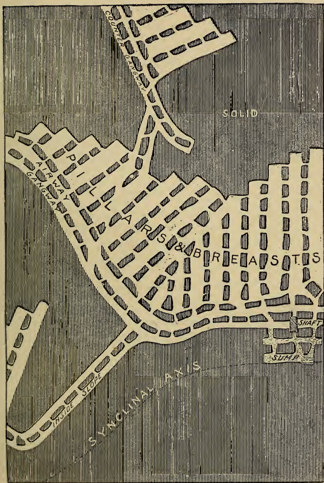
PLAN OF AN ANTHRACITE MINE WITH A SHAFT ENTRANCE.
