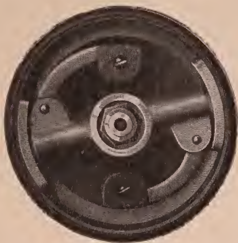
Fig. 222. Governor of Auto-Lite Permanent-Magnet Type Generator
