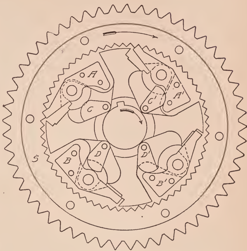
Fig. 161. Ratchet and Pawl Type Overrunning Clutch ( Horseless Age )
