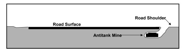
Figure 3-11. Buried Pressure Mine
