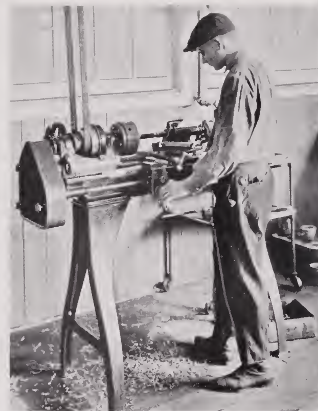
SENEGA FALLS 9-INCH ENGINE LATHE
