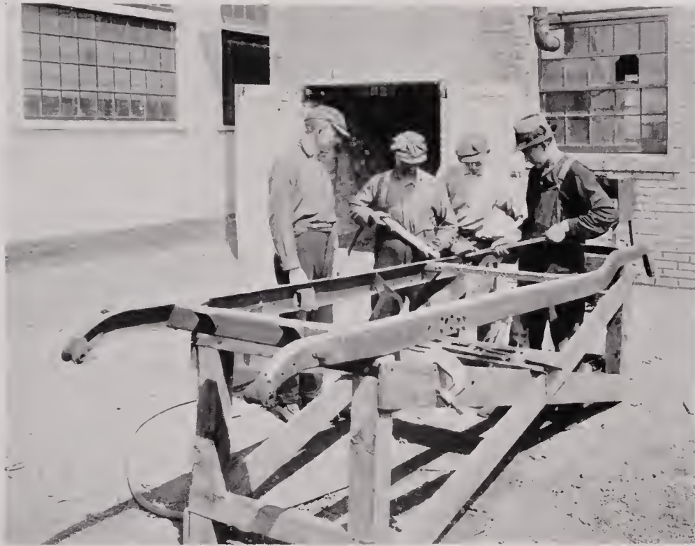
RIVETING MODEL 250 FRAMES
