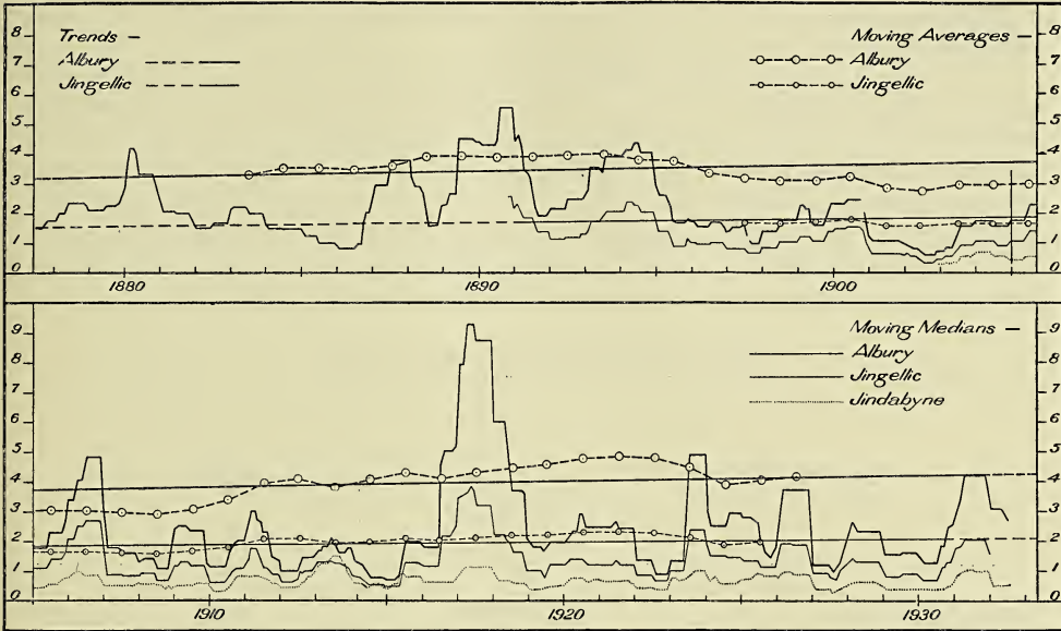
Text-fig. 6.—Fluctuations of the upper Murray and Snowy Rivers. The moving median with a 12-month period, plotted monthly, eliminates the annual wave: the 13-year moving average of annual totals eliminates the minor cycles, and the computed trend gives the secular movement of volume. For the medians, ordinate numbers are multiplied by 100,000 acre-feet: for the averages and trends, by 1,000,000 acre-feet. Scales are thus in the ratio—median:average=12:10.
