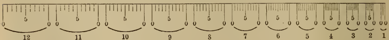
Figure 32, which may be designated as the scale of decimal parts , gives a series of spaces (millimeters as indicated by the
