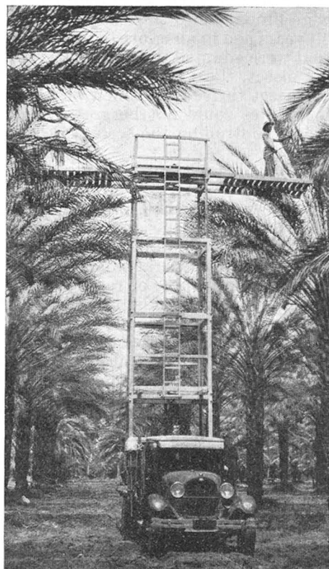
FIGURE 48.—Truck and tower for inspection of tall date palms for presence of the Parlatoria date scale.
