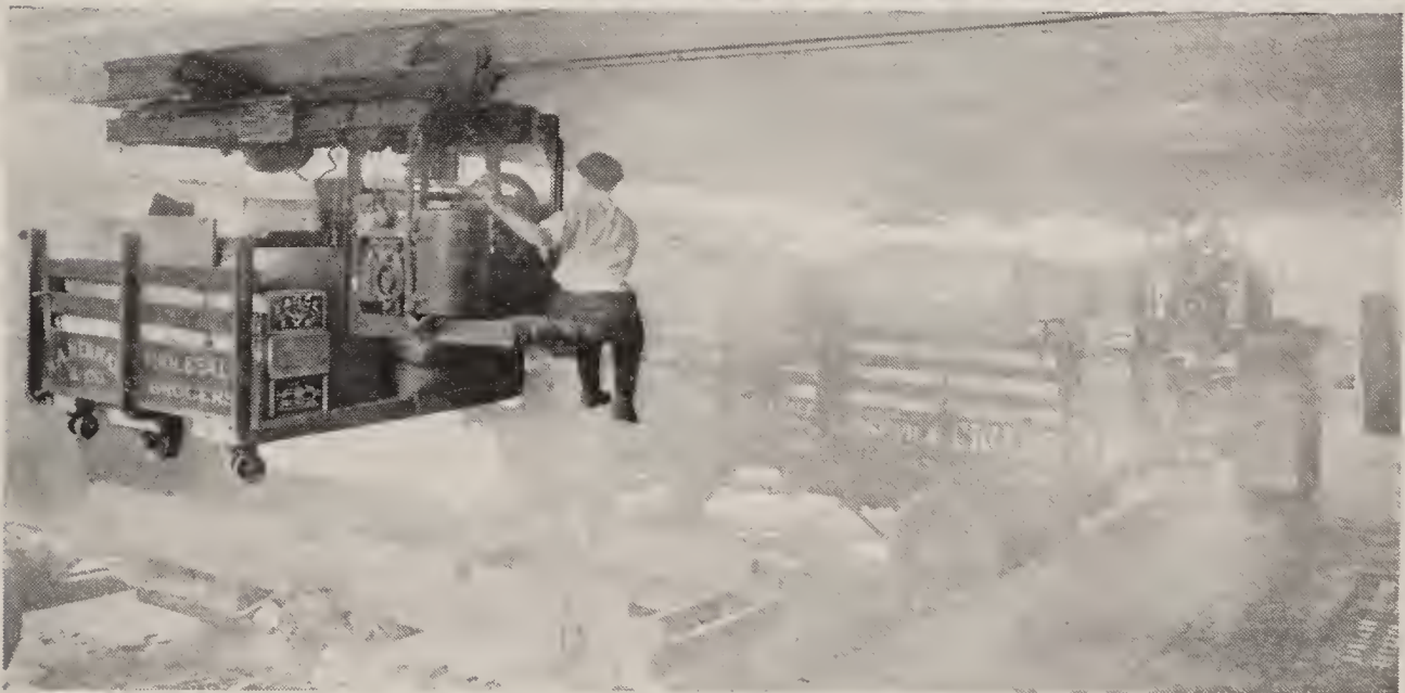
Cranes are not limited to handling large, bulky articles. Small articles grouped also may be so handled to advantage (top). Special slings enable a crane operator unaided (middle) to pick up twenty-ton tractors. At the M. A. Newmark Company (bottom), a monorail carrier picks up and transports loaded trucks, which also serve as auto-truck bodies
