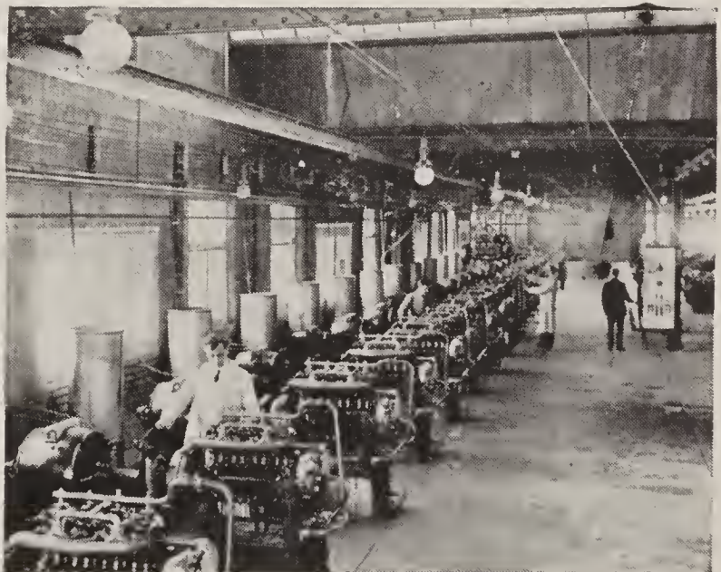
Permanently wired tables and a portable test-instrument desk (lower left) permit small motors to be tested together. Another company (lower right) uses dynamos in a similar group test, and pumps the current into the power mains. Direct reading scales and beam scales in the open (left above), stock bins on wheels and galvanized iron lockers for stock (right) cut costs
