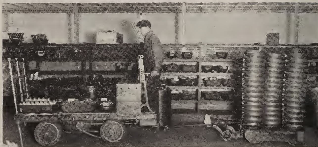
Magnet-lift attachments on cranes greatly increase their efficiency. The one shown (upper left) does the work of twenty men. Swivel cranes, easily shifted, serve groups of machines (upper right). Core-oven operation in a car-wheel plant is facilitated by rack cars and a transfer platform (middle). Industrial motor trucks have largely supplanted hand trucking at the Pierce-Arrow Motor Car plant.
