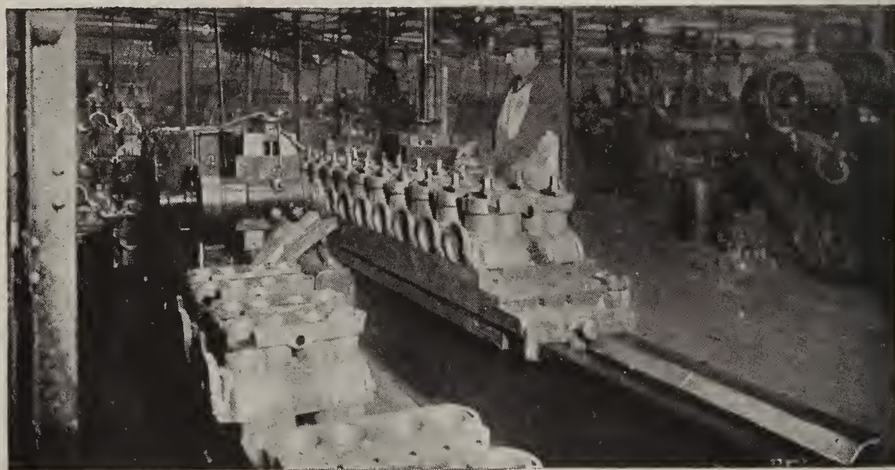
At the Packard Motor Company machine time is cut by a trackway for quick transfer of articles under successive multiple drill presses (top). Planing identical parts in groups rather than singly (bottom) is a Ford method. At the Westinghouse plant pneumatic fingers lift and hold the metal. Mechanical counters and air-ejection increase the output of the inclined punch presses at the right
