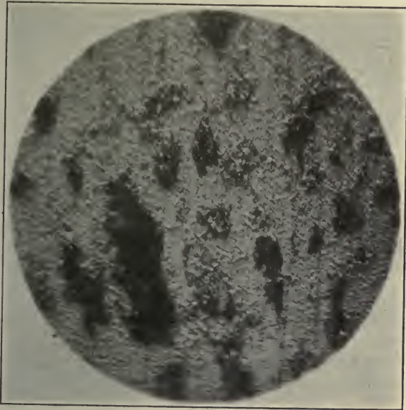
FIG. 71.—31-Minute Steam Activated Charcoal. Magnified 732 Diameters.
