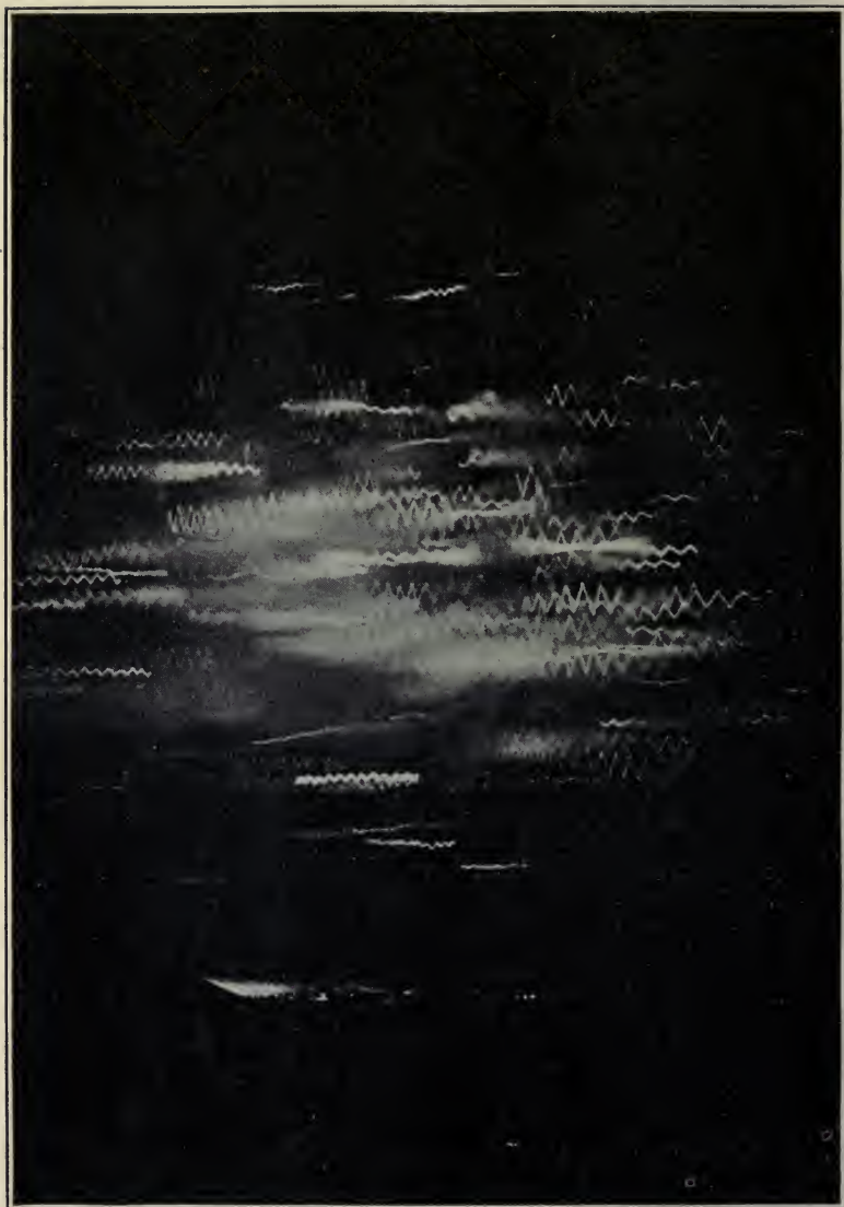
FIG. 88.—Measurement of Smoke Particles by Use of Ultramicroscope.
