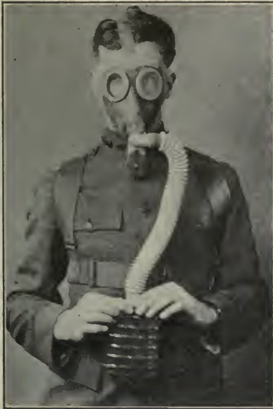
FIG. 66.—Ammonia Mask, Showing Relative Size of Canister.
