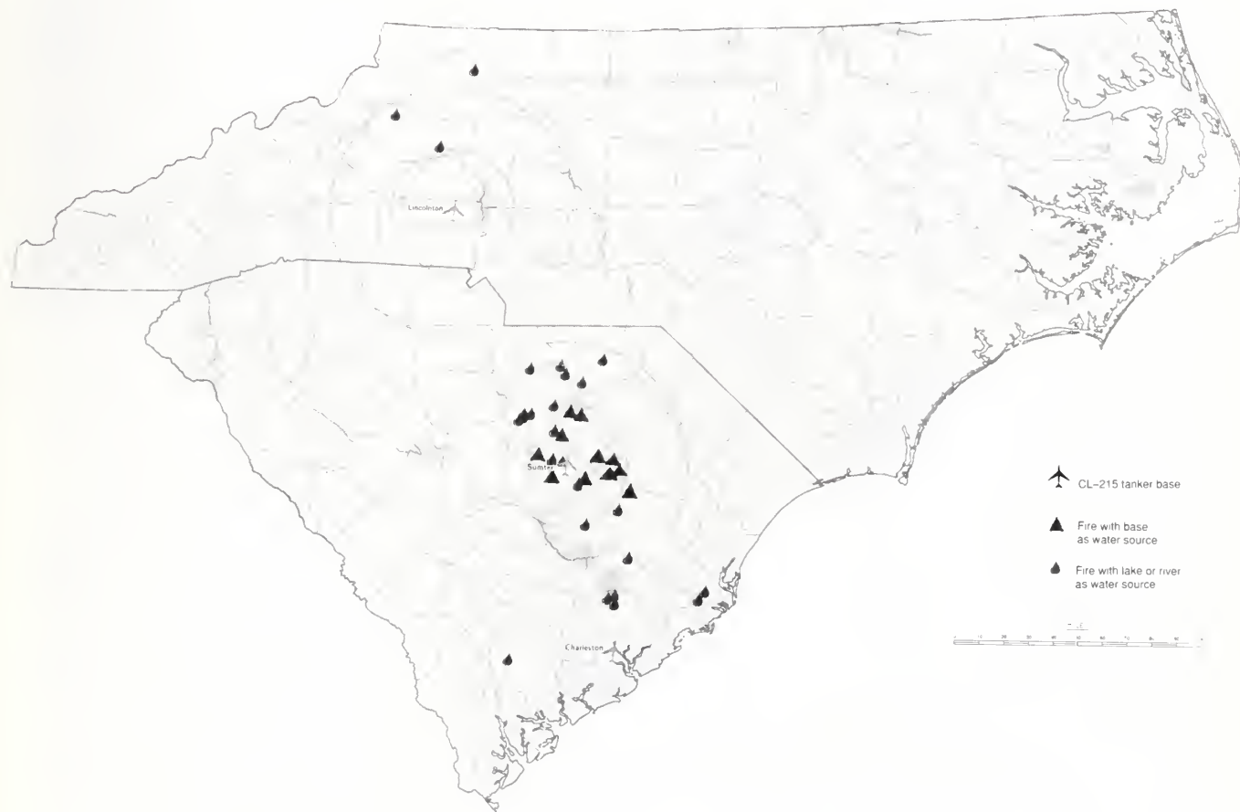
CL-215 tanker base map. (Notes: Water available for helicopters within 1 mile (1.6 km) of all fires. Scoop mode used on 26 fires (60%). Tanker base used as water source on 15 fires (40%). Average distance of suitable water source: CL-215—17 miles (27 km); helicopter—1 mile (1.6 km).)
