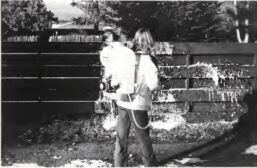
Lynn Bleeker, Payette National Forest engine foreman, demonstrates the use of power backpack pump.
