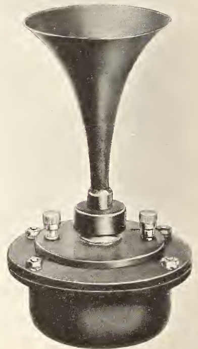
Electrodynamic speaker with horn, recently brought out by Racon Electric Company, Inc., of New York. Designed to cover frequency band from 3,000 to 10,000 cycles. Field rating, 6 or 110 volts, as specified. Voice coil impedance, 15 ohms. Height, 6¾ inches. Horn bell, 3 inches. Weight, 3 pounds.
