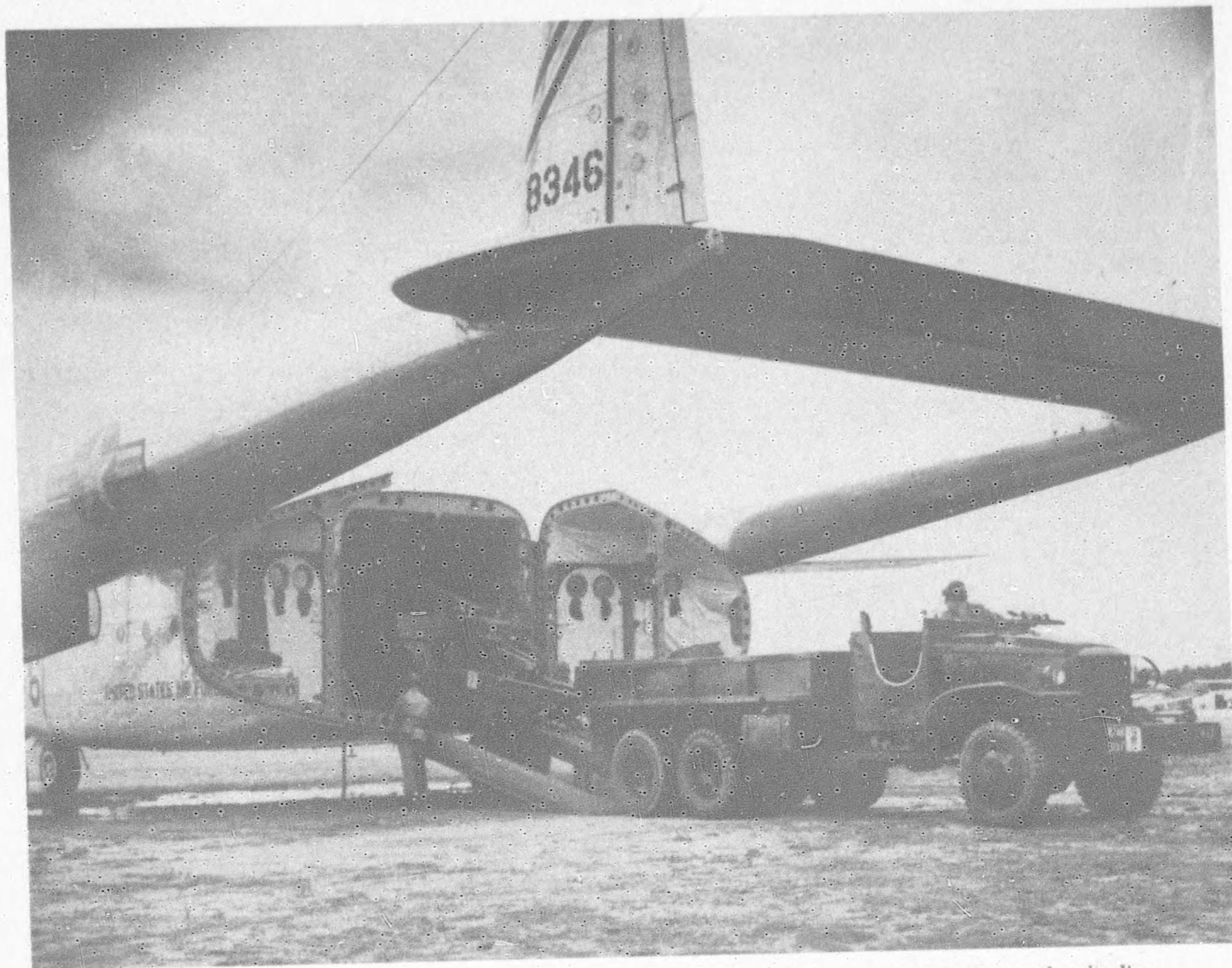
Among the favorable characteristics of the C-119 transport are its facilities for rapid loading and unloading.
