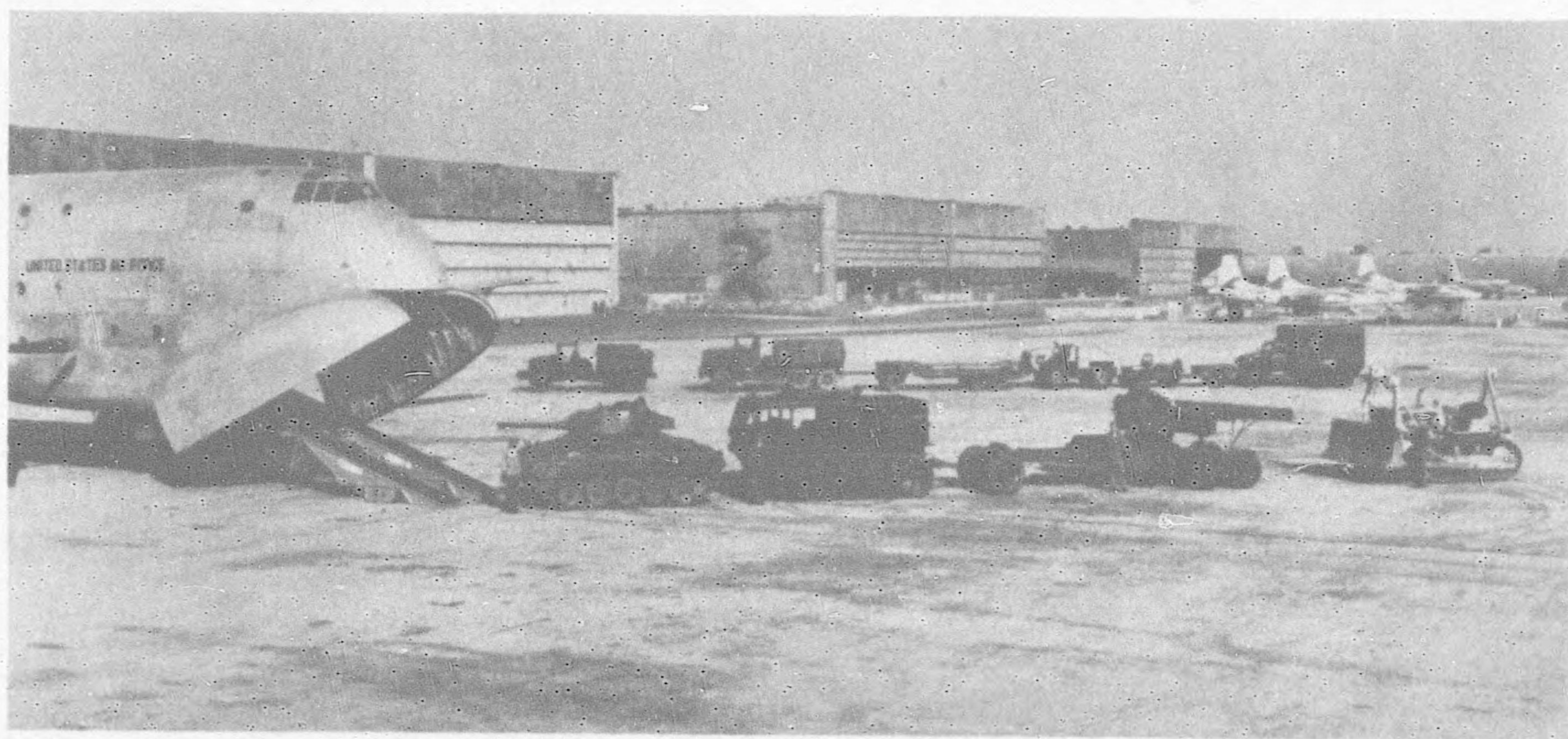
The C-124A can carry 94 percent of all military vehicles fully assembled and has facilities for rapid loading and unloading.
