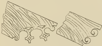
MOULDED ENDS OF ROOF TIMBERS FROM ADJOINING HOUSES
