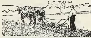
HARROW, McCORMICK-DEERING, SPRING TOOTH, WITH LEVERS
