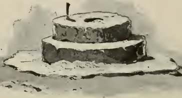
A HANDMILL FOR GRINDING CORN.— Nam. xi. 8.
