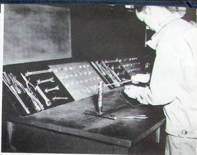
Mockup, Turnbuckle Safetying.
