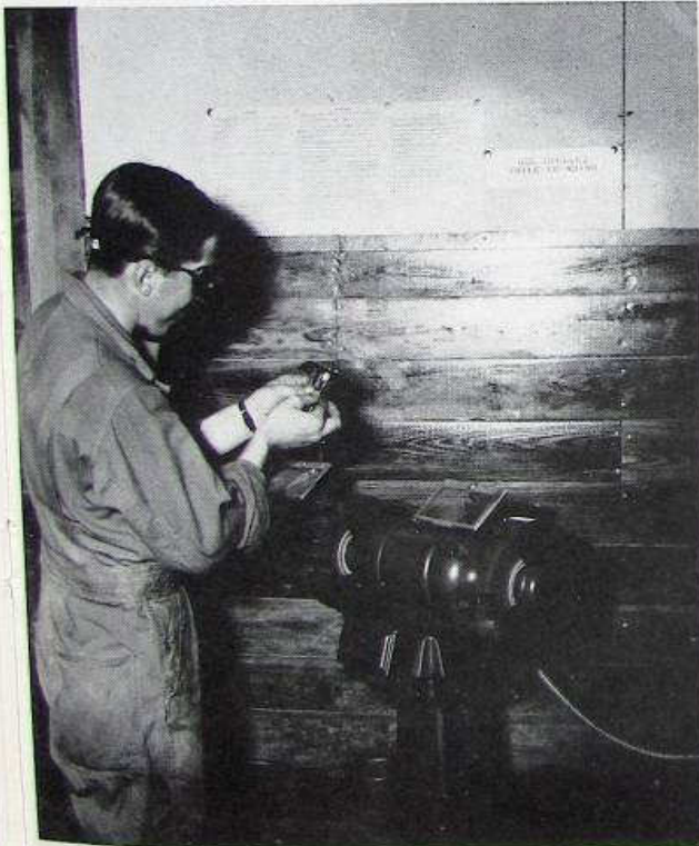
Drill Pitch Checking.
