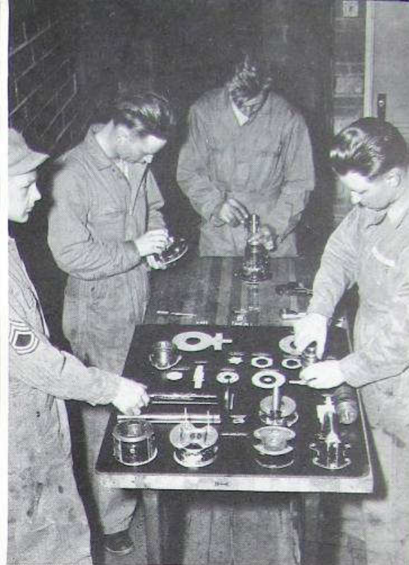
Starter-Energizer Parts Rack.
