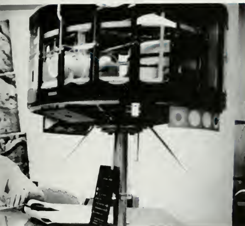
Edward Hach, A. T. & T. Long Lines sales representative, discusses the model with Robert Laudrille, NESC ground communications supervisor, to be sure facilities meet NESC present and future requirements. In foreground is a half-size scale model of the ESSA weather satellite, which permits working parts to be viewed.
