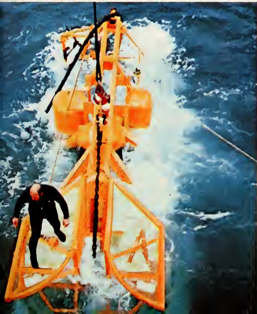
Television views of the plow at work were taken by three cameras on the plow and seen on screens in the ship's control room.
