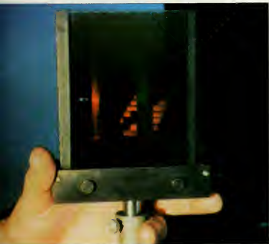
Recording specks and whirls on the holographic plate (above) record the pattern produced by the interaction of two laser beams. When illuminated by a beam of light (below), the original subject is recreated in a three-dimensional image which "floats" either before or behind the hologram.
