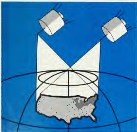
Initial phase of AT&T's proposed Space/Earth System calls for two satellites intermixed with ground facilities.
