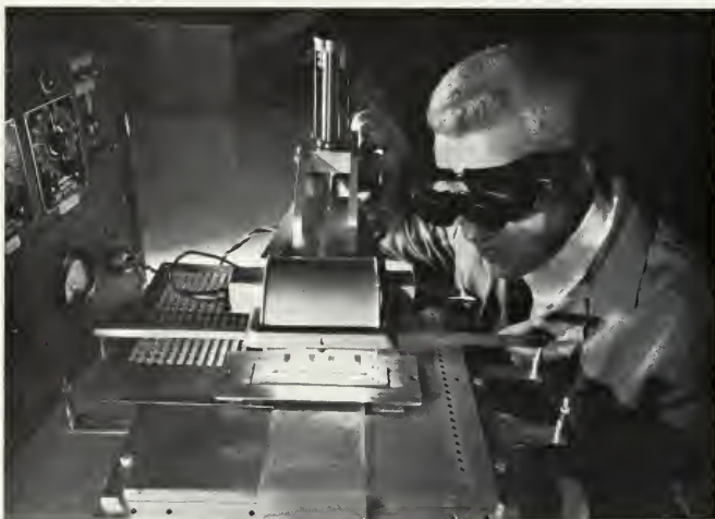
A. P. Boyer of Bell Labs inspects new infrared soldering device as it bonds flexible cable to printed circuit board. With this process, 50 or more connections can be made simultaneously.
