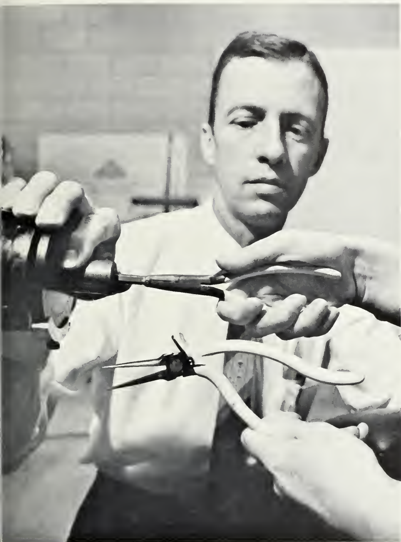
Western Electric biomechanics engineer studies bent wrist position caused by shape of conventional pliers. Contour handles and thumb stop of redesigned tool reduced strain.
