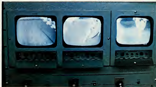
Television views of the plow at work were taken by three cameras on the plow and seen on screens in the ship's control room.
