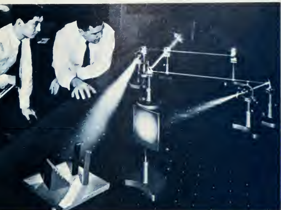
Bell Laboratories' Larry H. Lin (left) and Ken Poole make the multicolored hologram which is seen on the preceding page.
