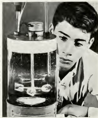
This small tank is a precision apparatus which enables students to grow crystals in the classroom. Crystallography is one of the subjects covered by Bell System science aids.
