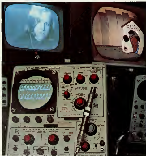
The shape of things to come: the oscilloscope shows the actual pulses in a stream, operating at 224 million bits per second, and carrying two television programs at once.
