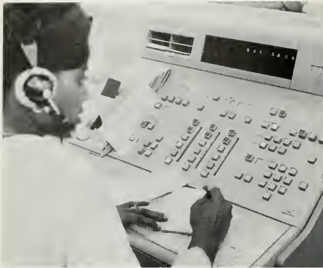
New traffic service positions reduce the time an operator spends on a call since equipment handles routine phases of a call.
