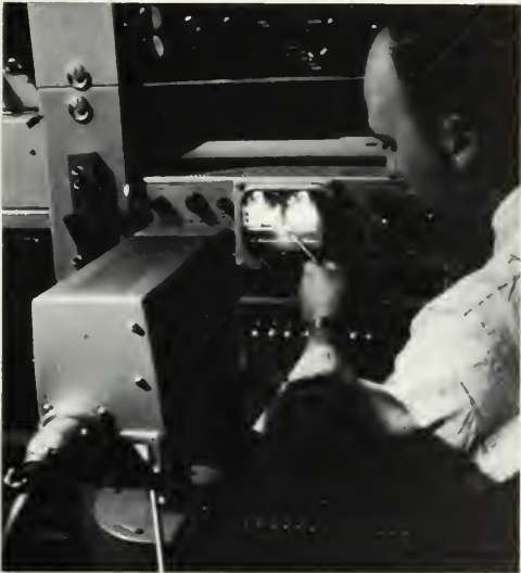
Beginning at remote pickup point, Bell technicians monitor signals. New device (above) shows each switching center quality of signal received, pinpoints trouble fast.
