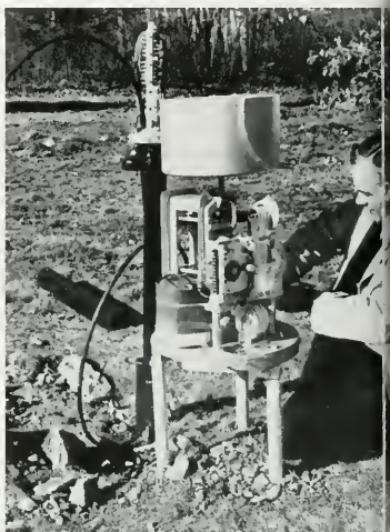
At Washington National Airport, left, data is relayed from Western Electric-designed equipment to meteorologist at map in Weather Bureau Control room. Information comes from 20 automatic reporting stations where recording devices, such as precipitation-sensing device being connected to system at right, provide constant data on possible flood conditions.
