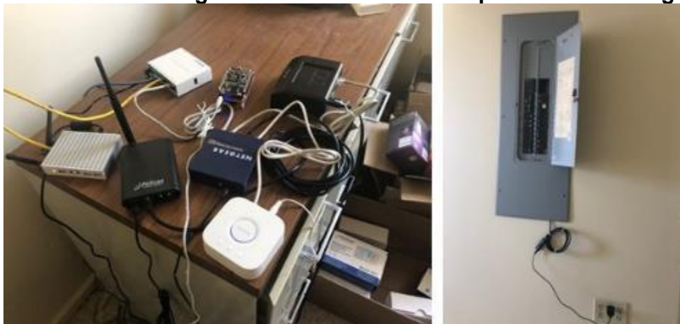
Figure 16: Installation of XBOS and Associated Devices for Building Energy Control and Management for XBOS-V Development and Testing
