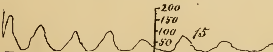
Lever rear-driver, 30-inch wheels, gear about 50; up hill, grade, one foot in twenty; continuation of No. 14, over top of hill.
