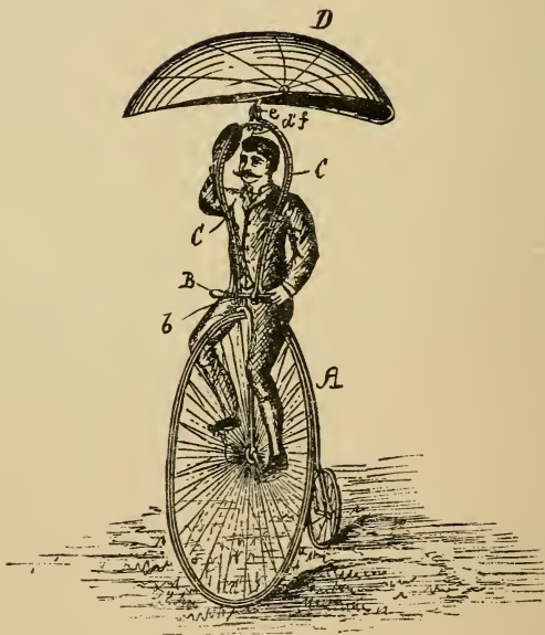
H. W. Libbey. Hood attachment for bicycles. No. 339,793. Patented April 13, 1886.
