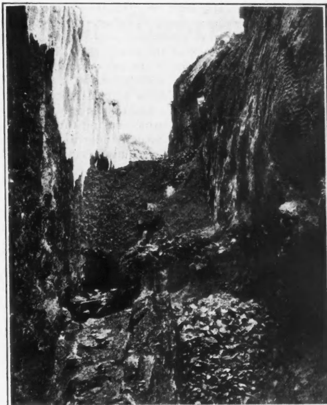
This vast artificial canyon was made by mining out a rich belt of ore. It is at the Bwana M'Kubwa mine, in Northern Rhodesia, and is 1,500 ft. long.
