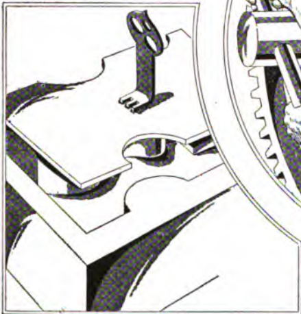
PUTTING A HANDLE ON THE TEMPLET HELPS IN FITTING
