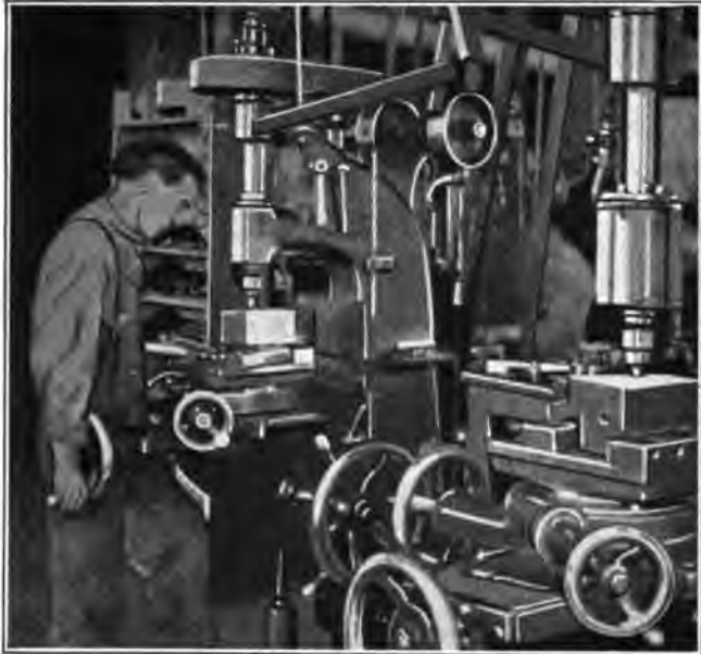
FIG. 2. SINKING RIFLE BOLT DIES
