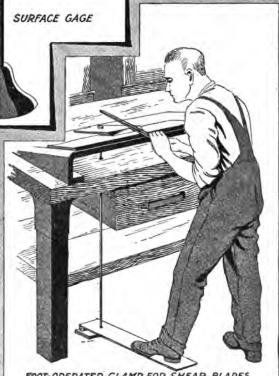
FOOT-OPERATED CLAMP FOR SHEAR BLADES
