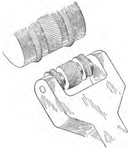
FIG. 9. HOLDER AND SPACING COLLARS FOR "BUILT-UP" KNURL
