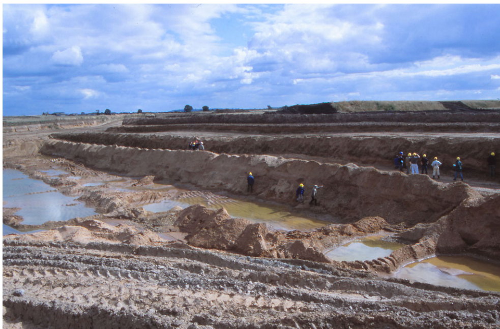
Figure 4. Section at the Finningley Quarry, looking southeast, September 2001. The base of the pit is in the ORG (unit 1), the working levels in Littoral Sands and Gravels (unit 4) and the upper level of the pit in the clay–silt of the Hemingbrough Formation (unit 5). Photo: P.C.B.
