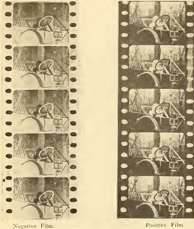
Fig. 20. Showing the difference between a negative film and the positive print taken from it. It will be noted that the light and dark portions of the negative are reversed on the positive.
