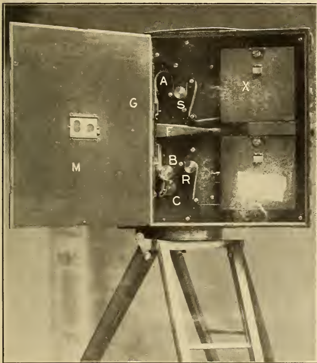
Fig. 18. The interior mechanism of a motion picture camera. F is the finder tube extending from the gate G to an opening in the back of the camera at Z. C is the intermittent claw movement. S and R are the feed and takeup sprockets that form the feed and takeup loops A and B respectively. X and Y are the feed and takeup reels. M is the access door.
