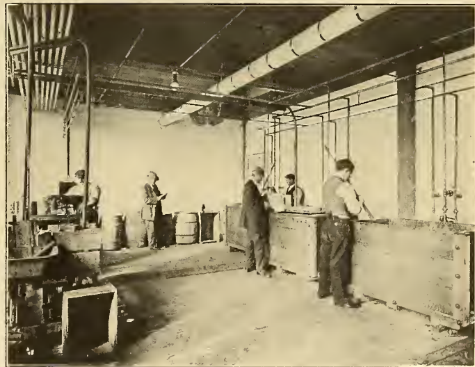
Fig. 23. Scene in a typical developing room showing the developing tanks.
