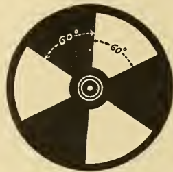
Fig. 9.—The Disc Shutter. Three Blades.
