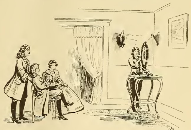
Fig. 3.—An Early Type of Disc Machine. The Pictures are Illuminated in Succession by a Narrow Beam of Light.
