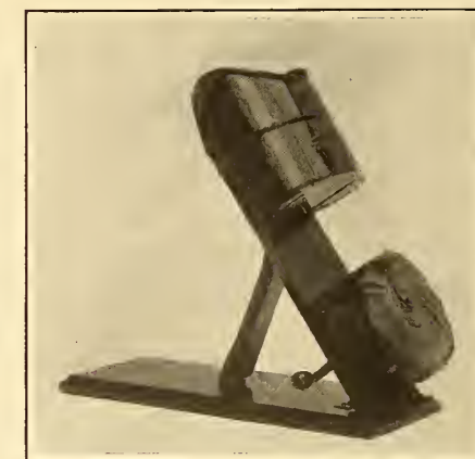
Fig. 7.—The Viewing Apparatus Showing Mounted Reel of Prints.
