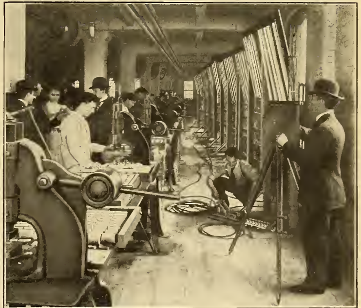
Fig. 29. Showing how an "industrial" film is taken in a factory. The rows of vertical tubes on the right of the picture are Cooper-Hewitt mercury vapor lamps used for illumination of the dark interior. A film of this nature has a great educational value in the motion picture theater, and is of great value to the manufacturer who wishes to have his customers become interested in the inner workings of his plant.
