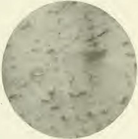
Fig. 4. Distorted Bearing Bronze, Magnified 100 Diameters. Un-etched
