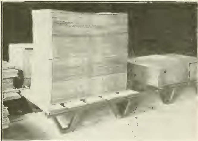
Steel Supported Truck Platform Loaded with Tin Plates to Capacity Greater than the Truck Can Lift to Show the Strength of Construction
