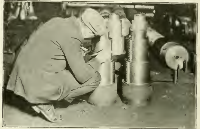
Fig. 5.—Crank Pins Are Calipered and the Dimensions Filled in on a Form.
