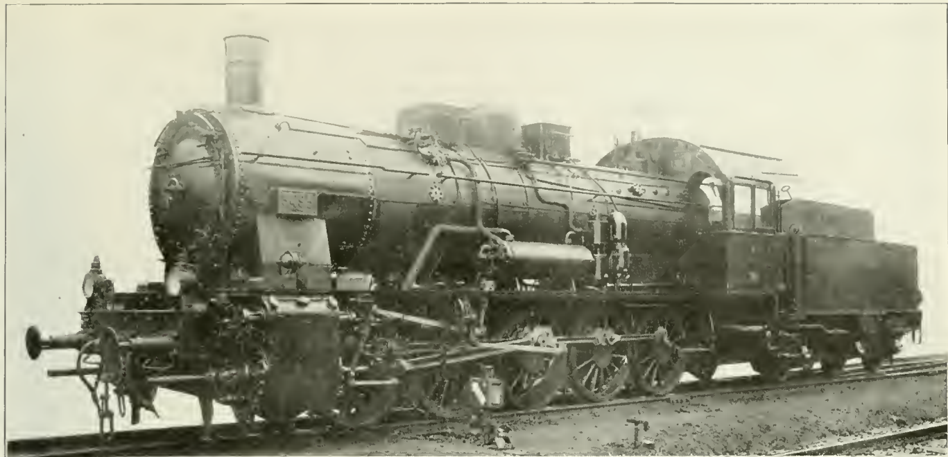
Superheater Freight Locomotives of the G-10 Type for the Prussian-Hessian Railway. The First Locomotive Built by Krupps.
