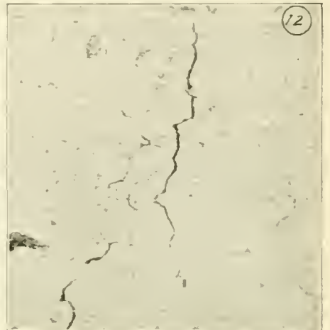
Fig. 6—Inter-granular cracks in strained oxy-acetylene weld. No defects visible before straining, showing that films were very thin.
