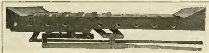
Side View of the Grate Showing the Operating Connections
