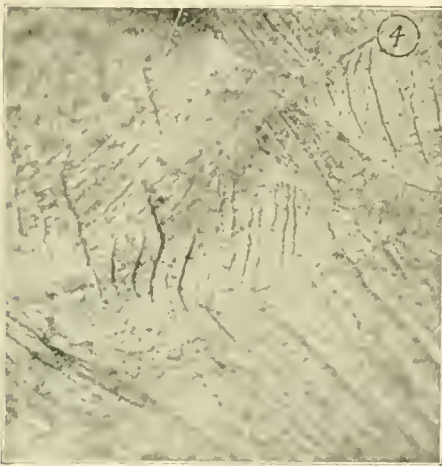
Fig. 1—Strained Iron. The curved lines are not cracks, but the edges of parts of the grains that have slipped past each other. They are called slip bands.
