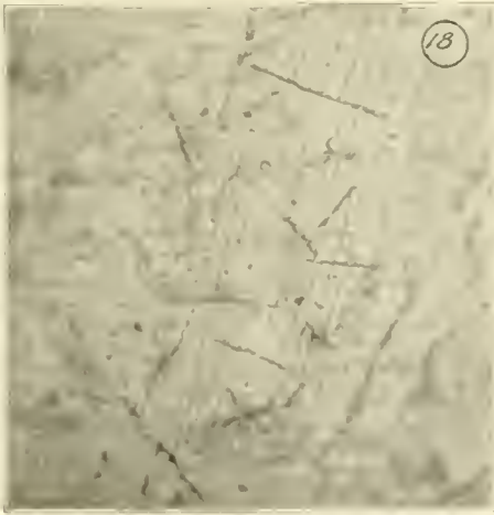
Fig. 8—Slip bands in arc weld. The heavier straight lines are iron nitride. These weaken the weld little, if any.
