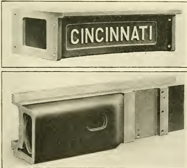
Fig. 1—Views Showing Box Section Construction of Planer Arch and Cross Rail
