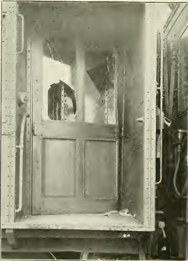
Rear End of Car, Showing Damage to Door in Collision
