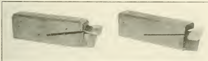
Tool Holder Designed for Use With Broken High Speed Steel Drills and Tool Bits
