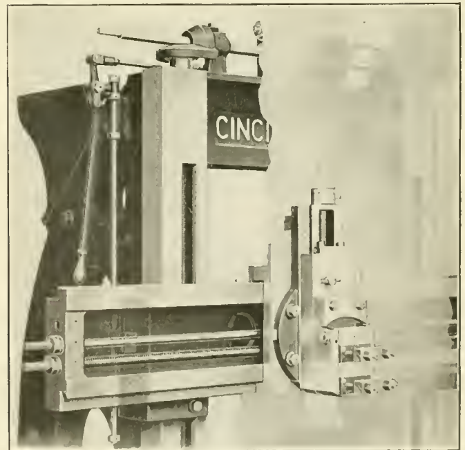
Fig. 2—Automatic Safety Stop for Elevating and Lowering Device
