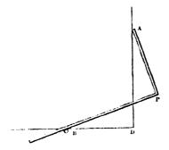
Let B be the fixed point. Then, if AP = BD, and the end A of the lever move along a straight line, while PC remains in contact with B, the cissoid is the locus of P.
