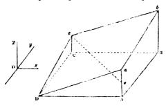
In the right-angled triangle aAD,  $aD^2 = Aa^2 + AD$ , (1.) Similarly,  $Dc^2 = DC^2 + Cc^2$ , (2.) To find the distance ac, let a perpendicular ce be drawn from c on to Aa. Then se = Aa - Cc, and in the right-angled triangle ace.
