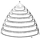
volume of the solid is the limit of the sum of a number of elementary cylinders having the same axis. Let  $\partial x$  be the altitude of one of these cylinders, y the radius of its base; x, y, y is the area of the base; and that area multiplied by the altitude, or x, y, y is the volume of the elementary cylinder. Therefore, the required volume is equal to
