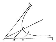
inclined to each other at an angle  $\alpha$ , as axes. Draw AB parallel to Oy, and let OB = c. The equation to the hyperbola is  $yx = c^2$ . Om = x.
