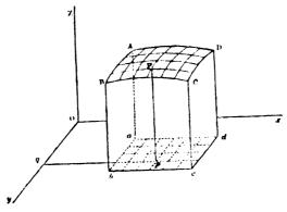
Let Pp be the altitude of one of the elementary parallelopipeds,  $\delta x$  and  $\delta y$  the length and breadth respectively of its base. Then the solid content of the parallelopiped is the product of these quantities, or  $z^3x\delta y = f(x, y)\delta x \cdot \delta y$ .
