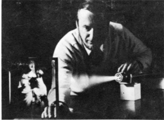
Dr. Wuerker aligns a ruby laser and holographic plate to recreate a three-dimensional image of a twelfth-century Madonna and Child, by an unknown Spanish sculptor.
