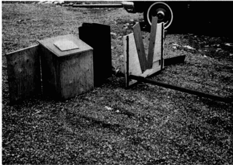
Figure 10 - Vee-Notches and Recorder for Flow Measurement
