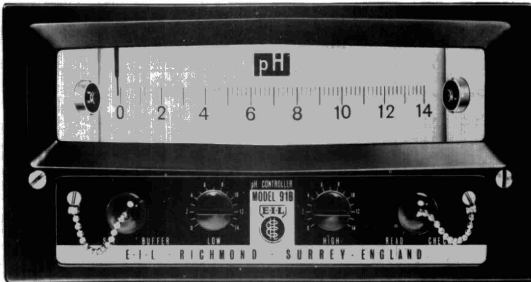
Figure 1 - a. Electronic Instruments Ltd. (England) Model 91B panel mounted pH meter-controller. The two control relays are electronically operated, and are adjusted by the controls marked "Low" and "High".
