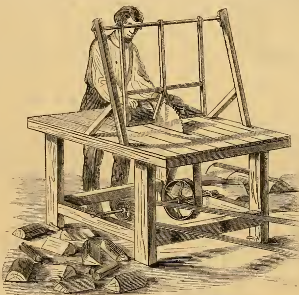
Fig. 2.—SAW WITH HANGING CARRIAGE.
