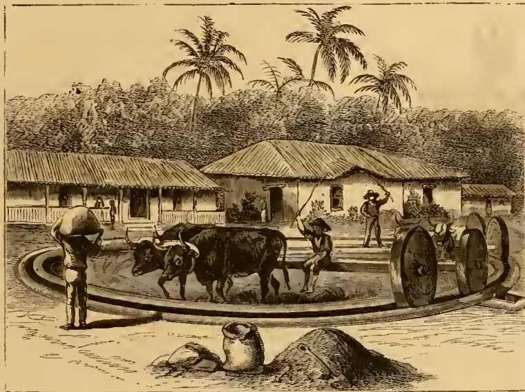
Fig. 4.—MILL FOR CLEANING THE COFFEE.
