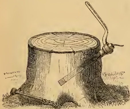
Fig. 1.—BLASTING WITH A SCREW-PLUG.
