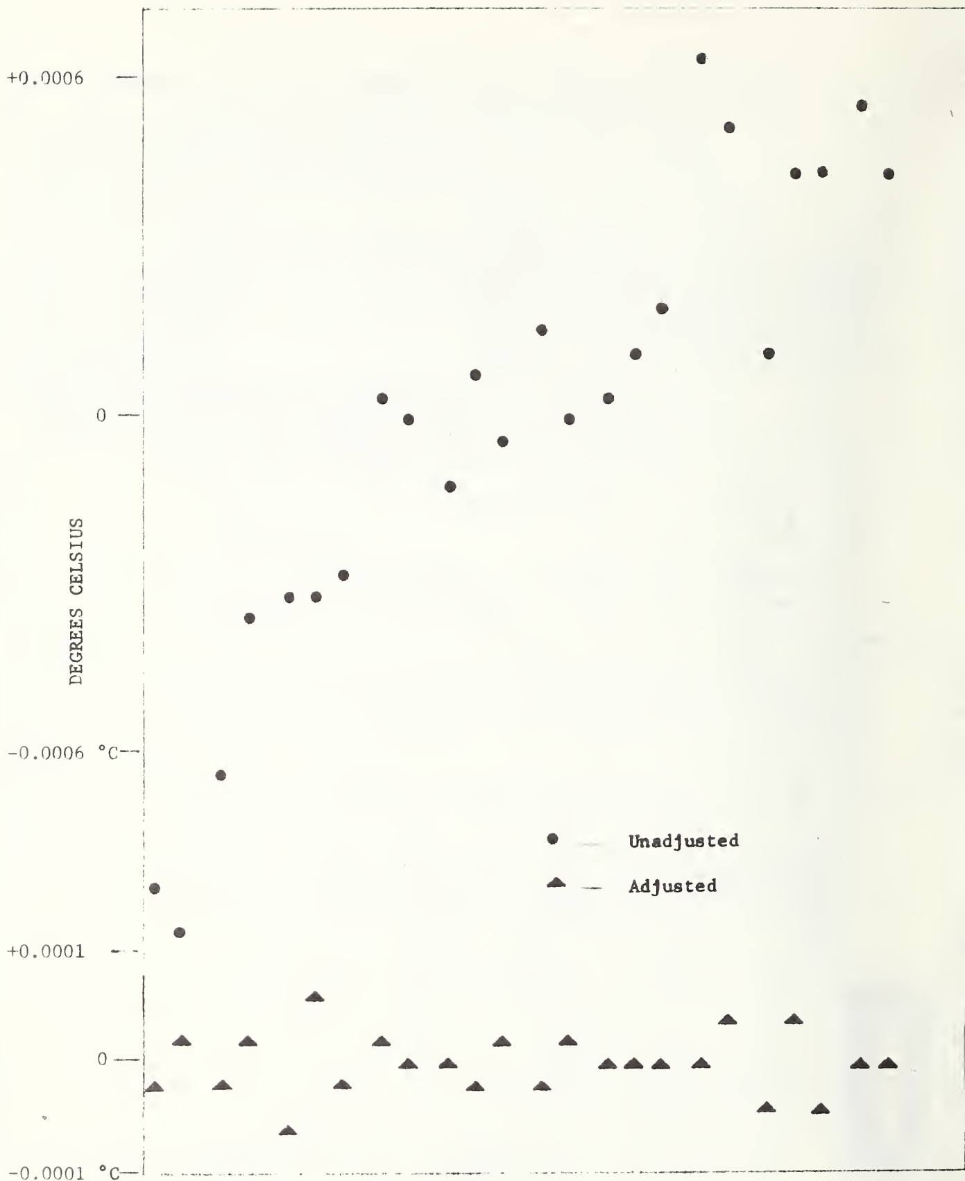
FIGURE 2: Plot of residuals illustrating behavior of bath at 15 °C during 50 minute interval required for the 24 observation series.
