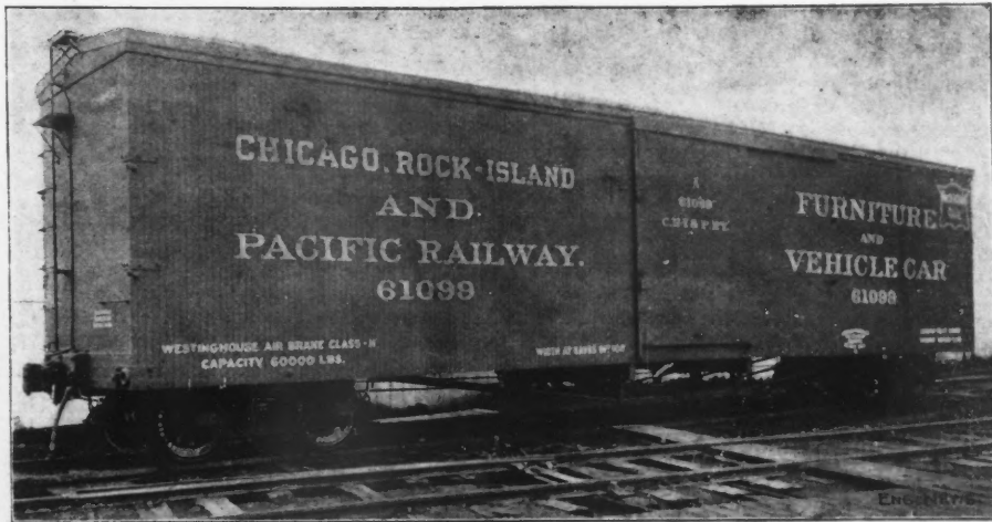
FIG. 1.—VIEW OF 50-FT. FURNITURE CAR; CHICAGO, ROCK ISLAND & PACIFIC RY. Michigan-Peninsular Car Co., Builders.
