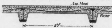
Fig. 1.—Section of Expanded Metal and Concrete Floor, for the New Refinery of the New York Sugar Refining Co., Long Island City, N. Y.
