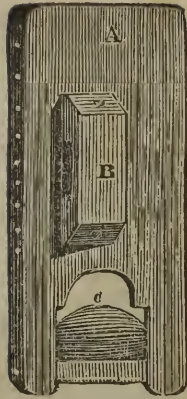
A, Splint. B, Cleat. C, Opening to ascertain the position of the heel.
