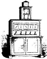
way apparatus, with its needles and handles; a separate wire and circuit being necessary for each needle. So few two needles however. have. been found sufficient to make all the requisite communications. The needle to the left is seen deflected one way. and that in the middle the opposite way. agreement must be made as to the meanings represented by each deflection or com-
