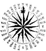
guide navigation in the open ocean, when there is no mark either in the sky or on the visible horizon to distinguish north, south, east, and west. By pointing always to the north, or within a known angle of the exact north point. it shows the course of the ship at every moment. The most essential part is a magnetised bar of steel, called the needle, which is supported horizontally on a central pivot, round
