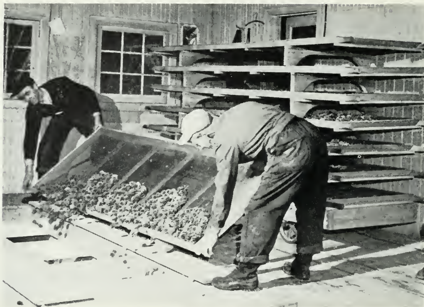
CONES ARE DRIED ON THE DRYING TRAYS AND EMPTIED INTO THE CONE SHAKER AT THE SEED EXTRACTION PLANT, ANGUS
