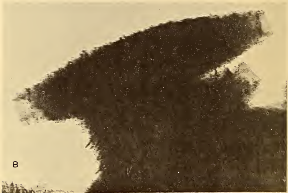
Fig. 15. Transmission electron micrographs of different aspects of similar polypropylene aggregates formed within nine hours of crystallizing the polymer from a 3/4% solution in amyl acetate at 115°C. (a) The aggregate is oriented with the plane of preferential development normal to the direction of viewing. (b) The aggregate is viewed parallel to the plane of preferential development. (x 30,200)
