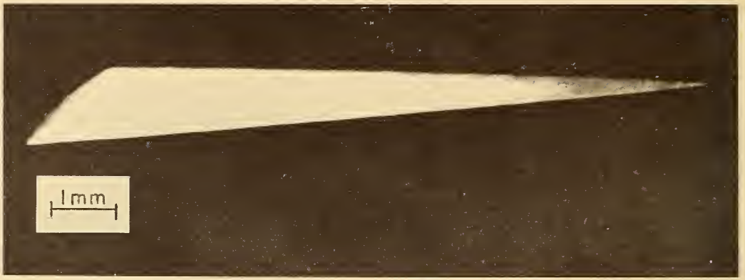
Fig. 1. Lang topographic photograph of the tip of an Al crystal with the axis parallel to [001] direction.
