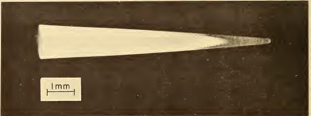
Fig. 2. Lang topographic photograph of the tip of an Al crystal with the axis parallel to [111] .
