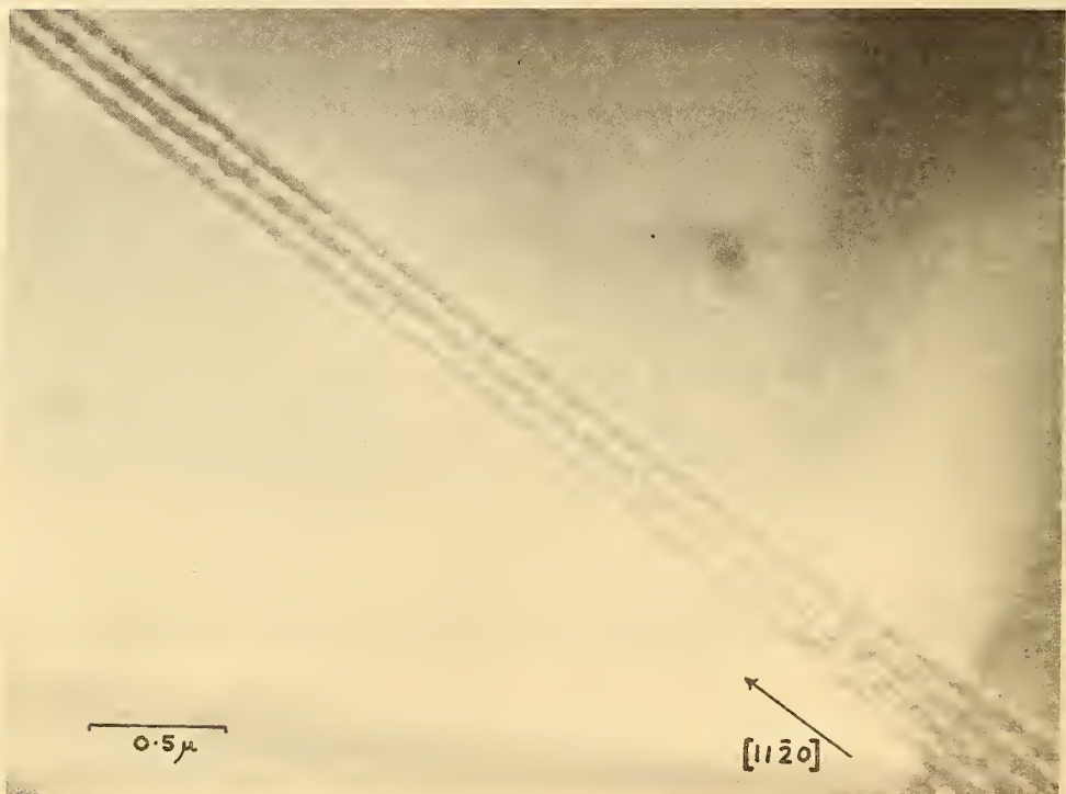
Fig. 19. Climbing dislocations in \alpha -Al 2 O 3 under the influence of a flux of point defects at \sim 1500^\circ\text{C} .
