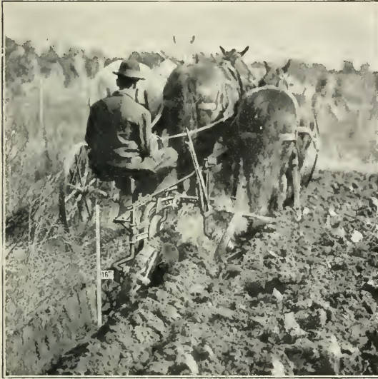
John Deere Deep-Tilling Stag Turning a Furrow 16 Inches Deep
