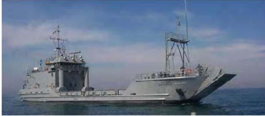
Figure 14. LCU-2000. It provides a slow heavy lift container or vehicle transfer to shallow water austere ports or beaches. (From U.S. Army Transportation Office, 2008, p. A-7)
