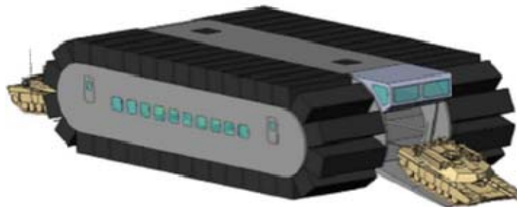
Figure 3. A modeling illustration of ONR’s UHAC. The UHAC supports multiple mixed load configurations and an unprecedented heavy load capacity. (From Main, 2010, p. 21)
