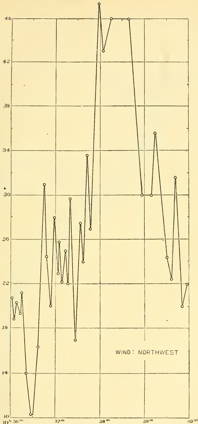
Wind velocities observed at Smithsonian Institution, February 20, 1893, with a Robinson anemometer (aluminum cups) registering every five revolutions.
