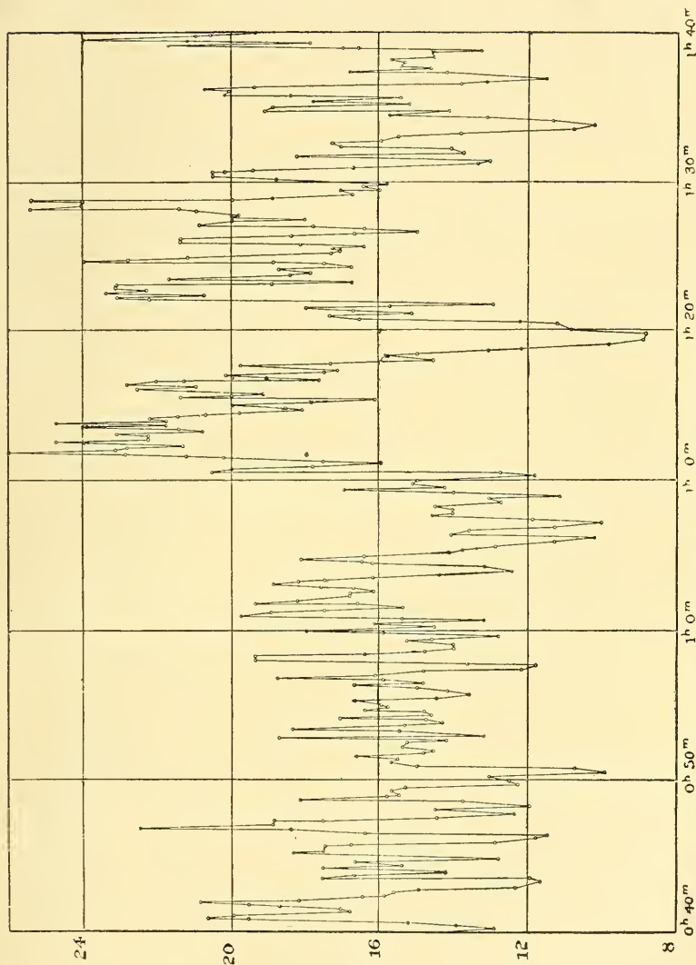
Wind velocities recorded July 16, 1887, at the Allegheny Observatory, with a Robinson anemometer registering every 25 revolutions. Abscissae = Time. Ordinates = Wind velocities in miles per hour.
