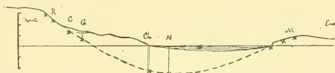
FIG. 2. Section across Seneca Lake at Geneva, from west to east, showing probable depth of buried channel. R, Reservoir; C, Castle Creek; G, Geneva Nat. Gas Spring Co.; Ch, Chase's well; N, Nester's well; M, outcropping of Marcellus shale.
