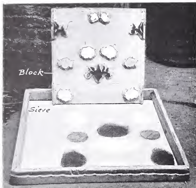
No. 7.—Sieve set out for "patching," and block charged with colour from it.
