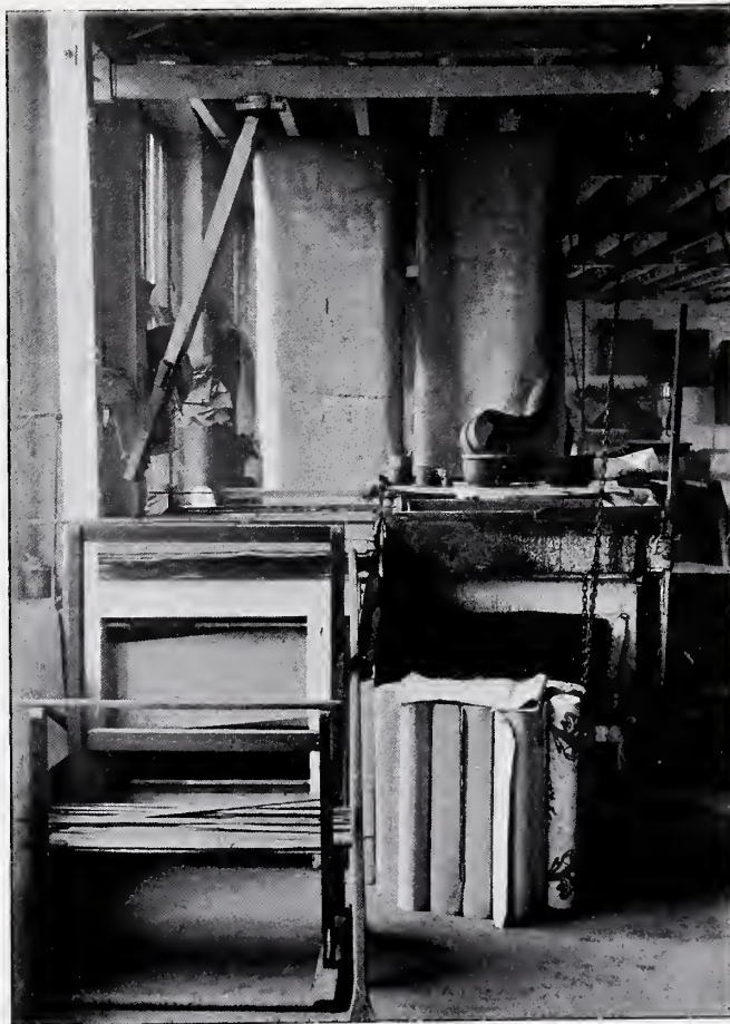
No. 2.—Block-printer's Table : pole above it; sieve to the right; beyond, paper hung up to dry.
