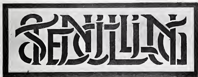
No. 1.—Stencil Plate of the elementary kind. The white represents the paper fret.
