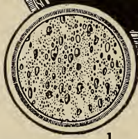
ILLUSTRATIONS No. 1 and No. 2 show in an enlarged way the difference in globules before (1) and after (2) being "cracked up" by the Chalmers Hot Spot.
